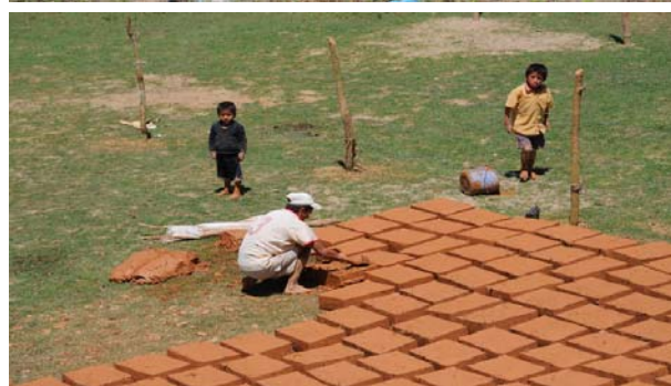
Fig. 3, 4. Preparation of construction materials (adobe) by the farmers themselves.
